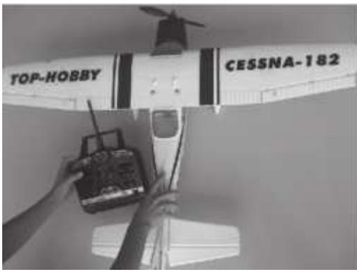
4. Please check the control surface and front wheel can work or not. Do not make it reverse, and make sure that the control surface & free wheel and the joystick are in the same direction.
